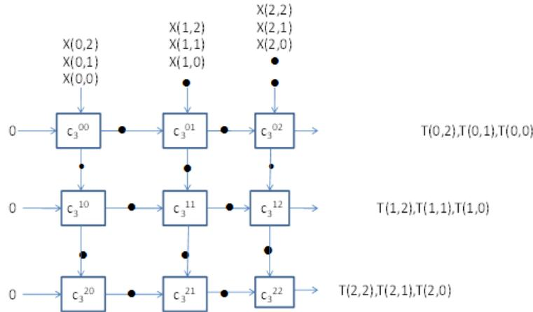
Fig.1. Systolic architecture for computation of  $T(k, n)$  given by (4) for  $N = 3; k = 0, 1, 2; n = 0, 1, 2$ .
