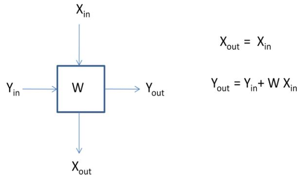
Fig.3. Function of each PE of systolic architectures shown in Fig.1 & Fig.2.
