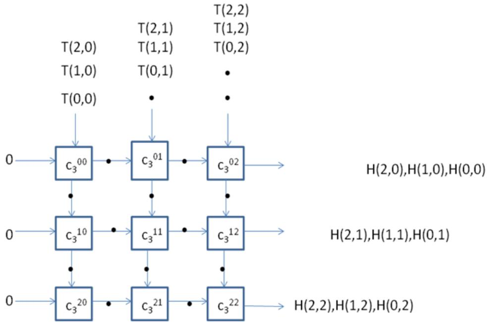
Fig.2. Systolic architecture for computation of 2-D DHT,  $H(k, l)$ , given by (5) for  $N = 3$ .
